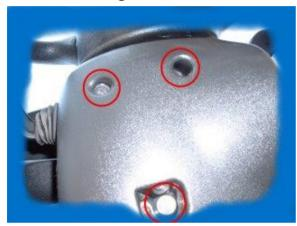
Below the ignition lock there are 3 screws which have to be removed
