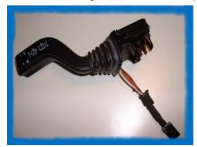
Replace the old windshield wiper switch with the new one. Just pull off the connector, then press the plastic lockings at the top and the bottom of the wiper. Now pull it out and replace them.
