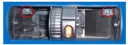
As soon as you have removed both grids, you can loosen the screws of the TID
